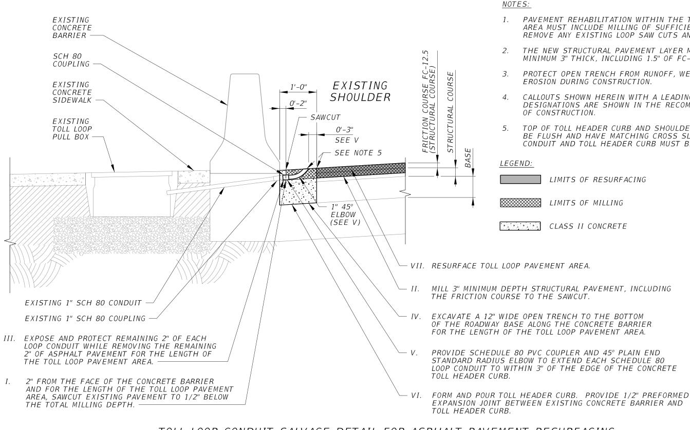
TOLL LOOP CONDUIT SALVAGE DETAIL FOR ASPHALT PAVEMENT RESURFACING
