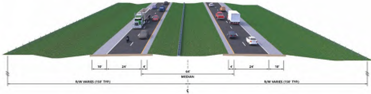
Figure 2: Existing Typical Section
