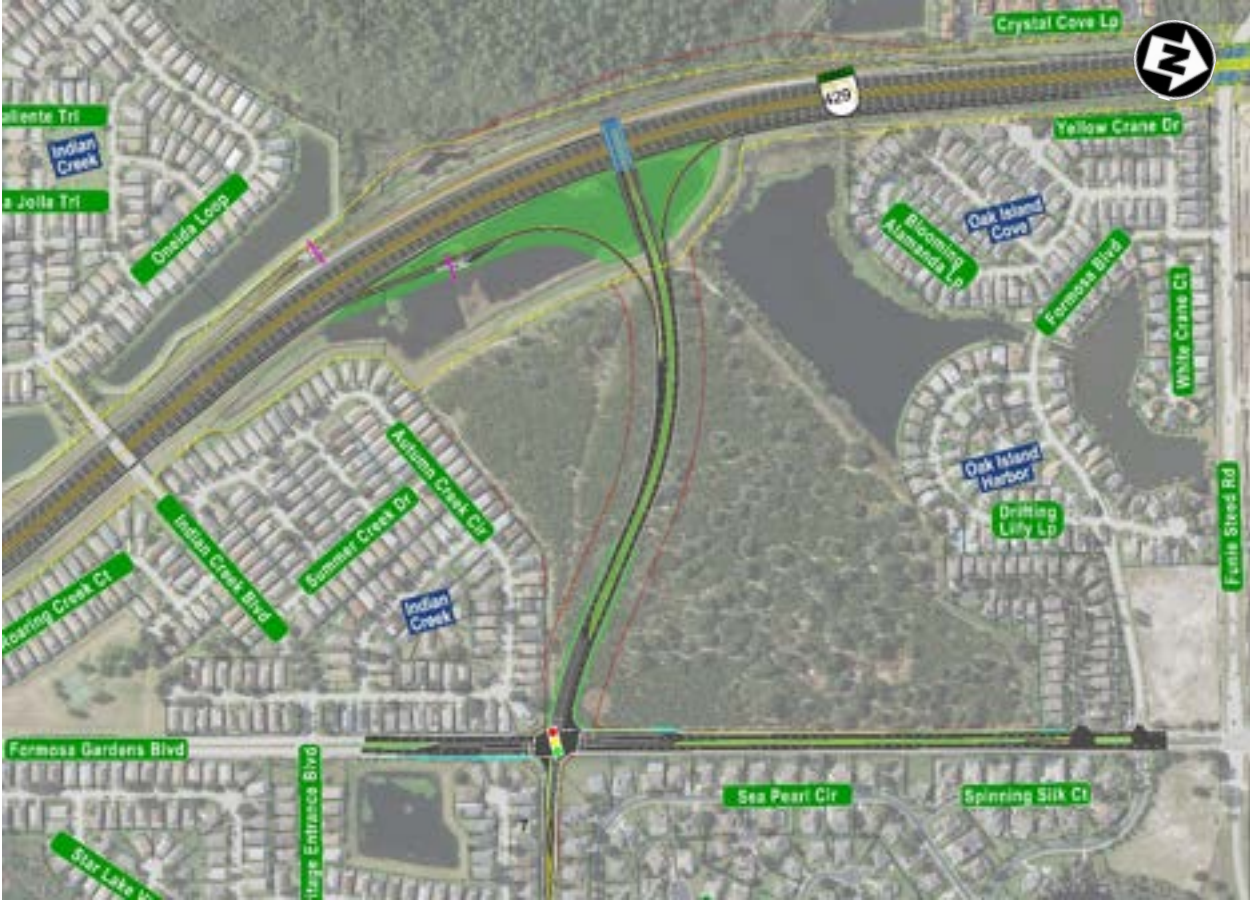
Figure 4-7: Livingston Road Interchange Alternative 2 T-Ramp Interchange
