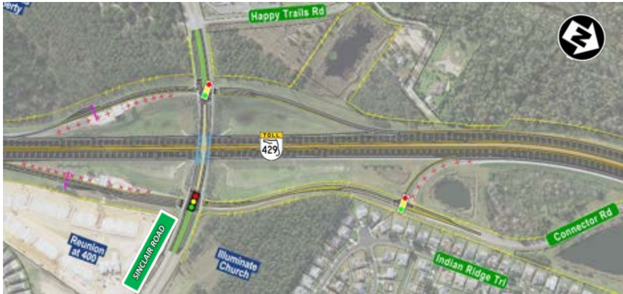
Figure 4-4: Sinclair Road Alternative 1 Traffic Signal
