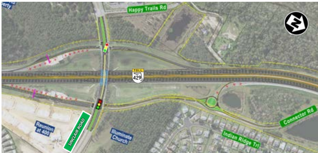
Figure 4-5: Sinclair Road Alternative 2 Roundabout
