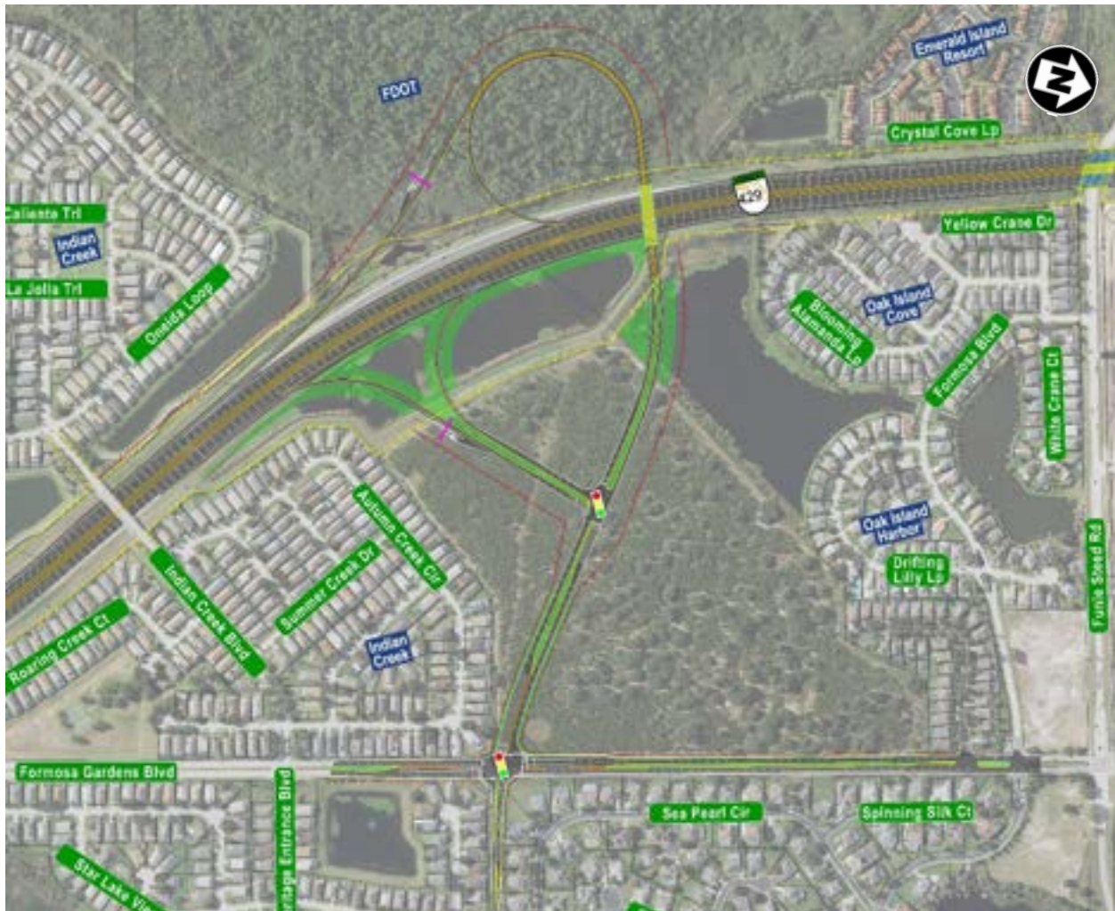
Figure 4-6: Livingston Road Interchange Alternative 1 Partial Cloverleaf
