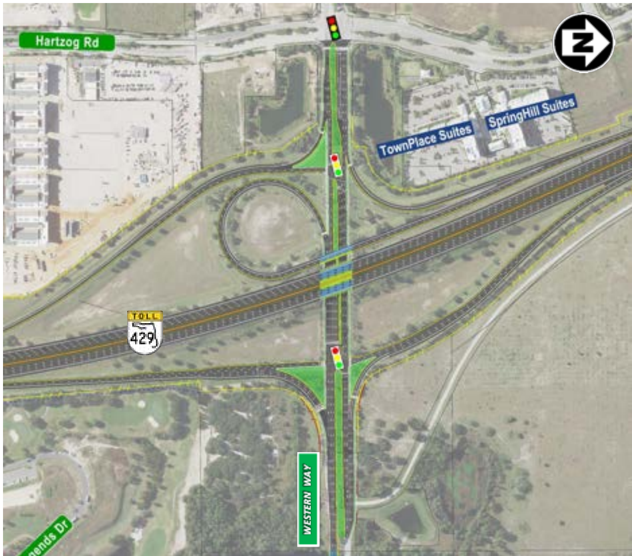
Figure 4-9: Western Way Interchange Build Alternative
