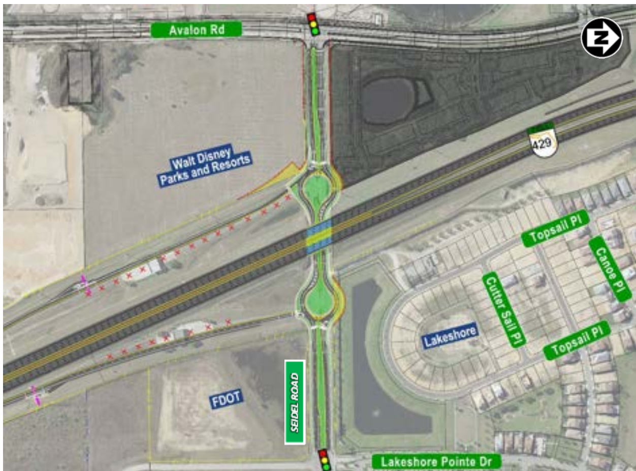
Figure 4-12: Seidel Road – Alternative 2 Double Roundabouts
