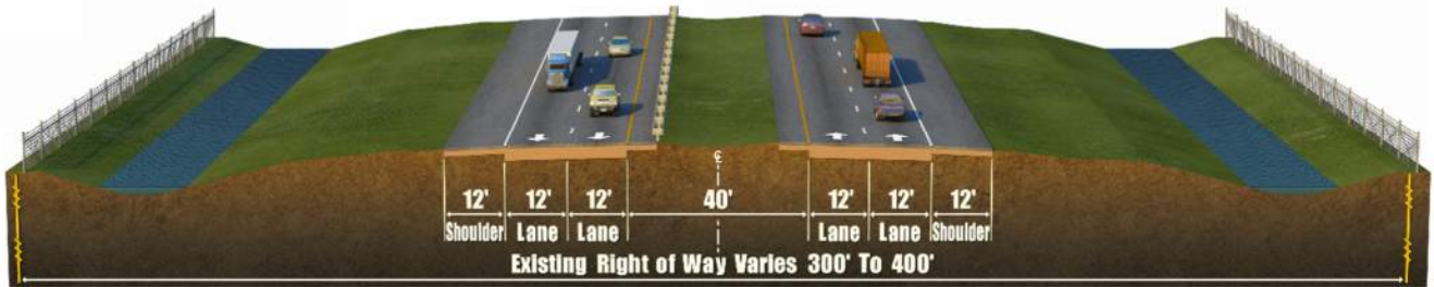
Figure 3-1: Existing Mainline Typical Section
