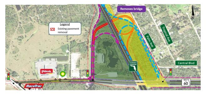
Osowou Road Emergency Access Improvements – Improvements to the existing Osowou emergency access includes replacement of the existing culvert and construction of a new 40-foot long bridge with 16'6" vertical clearance over Osowou Road and construction of a new northbound slip ramp. This will require raising the existing Turnpike Profile Approximately 5'6" for a distance of approximately 3,500 feet.
